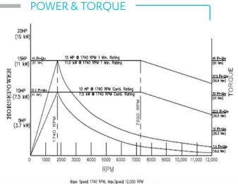
Nin. Power Roding/Torque Rating/Torque Rating - 10 HP (7.5 kH)/30.2 Ft-Lbs (41.0 Nm)
