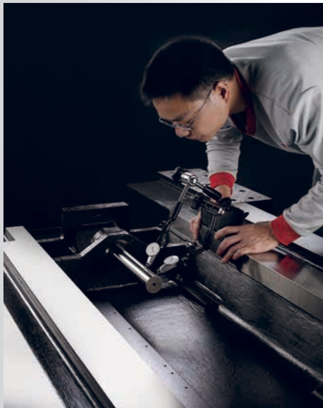
Hand scraped contact areas, minimal axis protection with maximum stroke.
